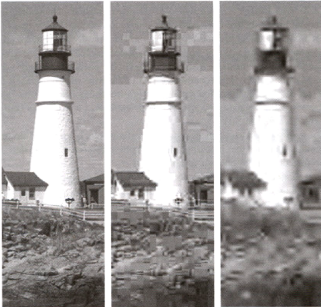
Figure 3-10 Illustration of artifacts due to compression (a) Original, (b) Block-DCT and (c) Wavelet, respectively. The blocking effect and staircase effect can be seen in b. Blur and ringing artifacts are seen in both the images (Winkler, 2004).
