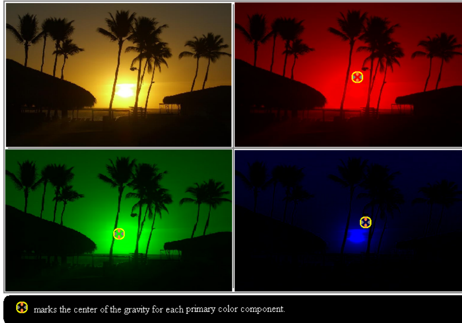
Fig. 3.9. Illustrates the center of gravities for each of the three color components in real life picture.
