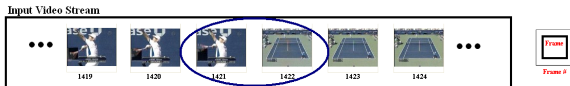
Fig. 2.2. Demonstrates an example for an abrupt transition (cut).
