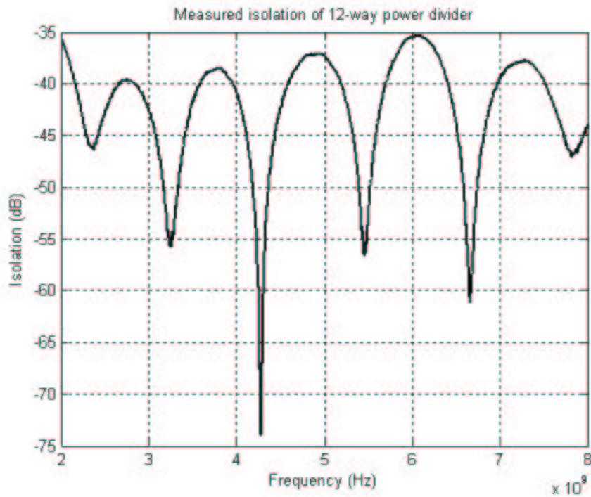
**Figure 5-1: Characteristics of 12-way power divider**
