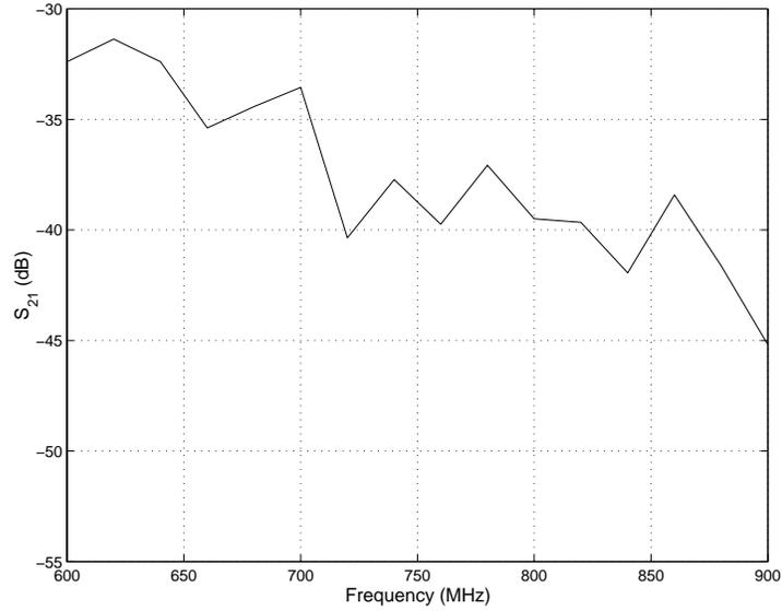
Figure 7.2. Transmission parameter ( $S_{21}$ ) between the horn antennas.
