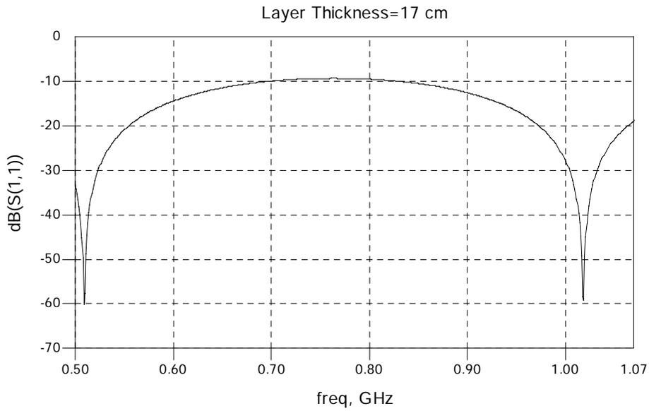
Figure 5.19. Simulated frequency response of reflection from a 17 cm layer.
