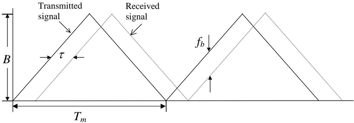
Figure 5.1. Transmit and receive signals from a point target for an FM-CW radar.  $B$  is the bandwidth of the signal,  $\tau$  is the two-way travel time from the radar system to the target,  $T_m$  is the modulation period and  $f_b$  is the beat frequency.
