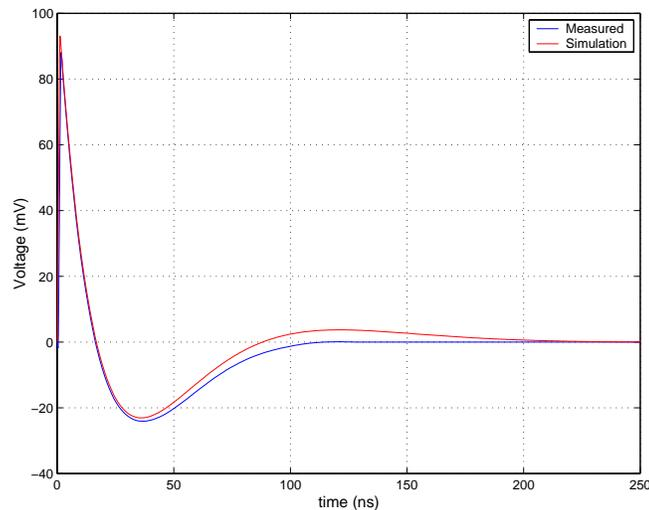
Figure 7.5. Comparison between measured and simulated responses to a 0.2 V step input.
