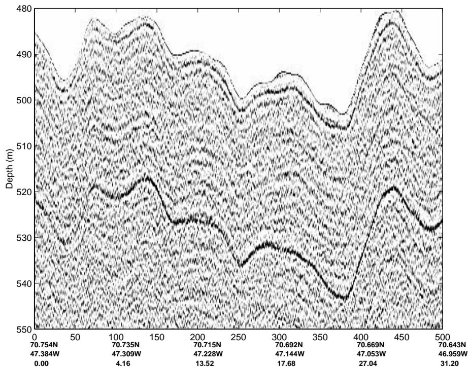
Figure 6.9. Internal layers observed at the wet snow zone of the icesheet.
