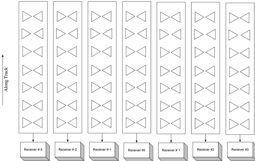
Figure 8.1. Bow-tie array to form beams digitally.
