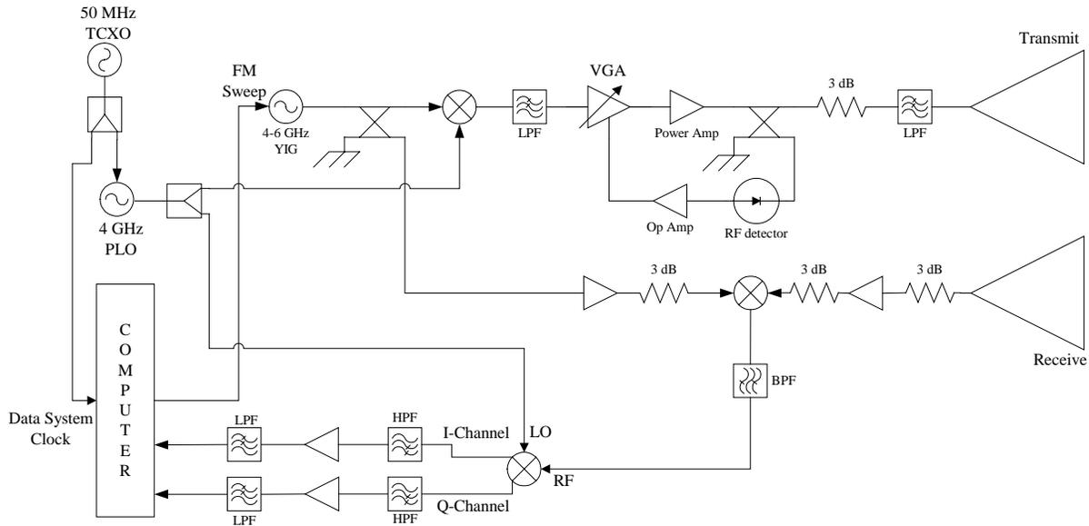
Figure 5.3. Block diagram of the prototype wideband FM-CW radar system for surface-based mapping of internal layers.
