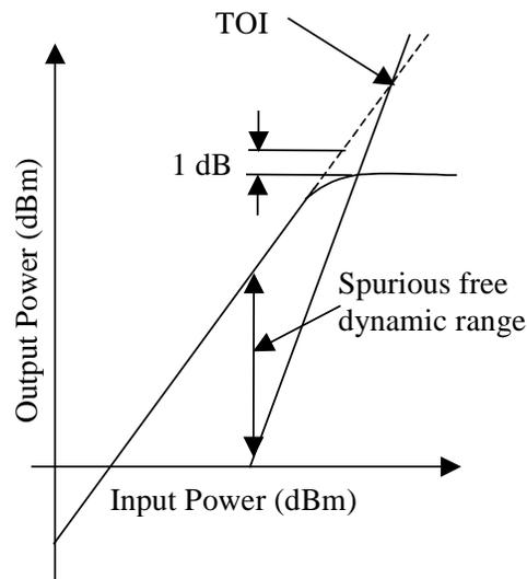
Figure 7.6. Illustration of 1 dB compression and third-order intercept points.
