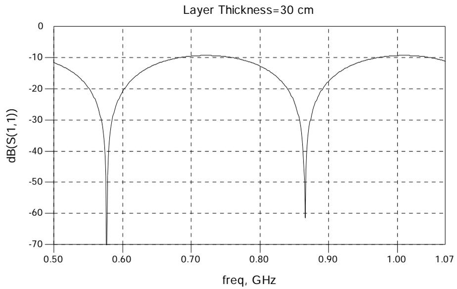
Figure 5.21. Simulated frequency response of reflection from a 30 cm layer.
