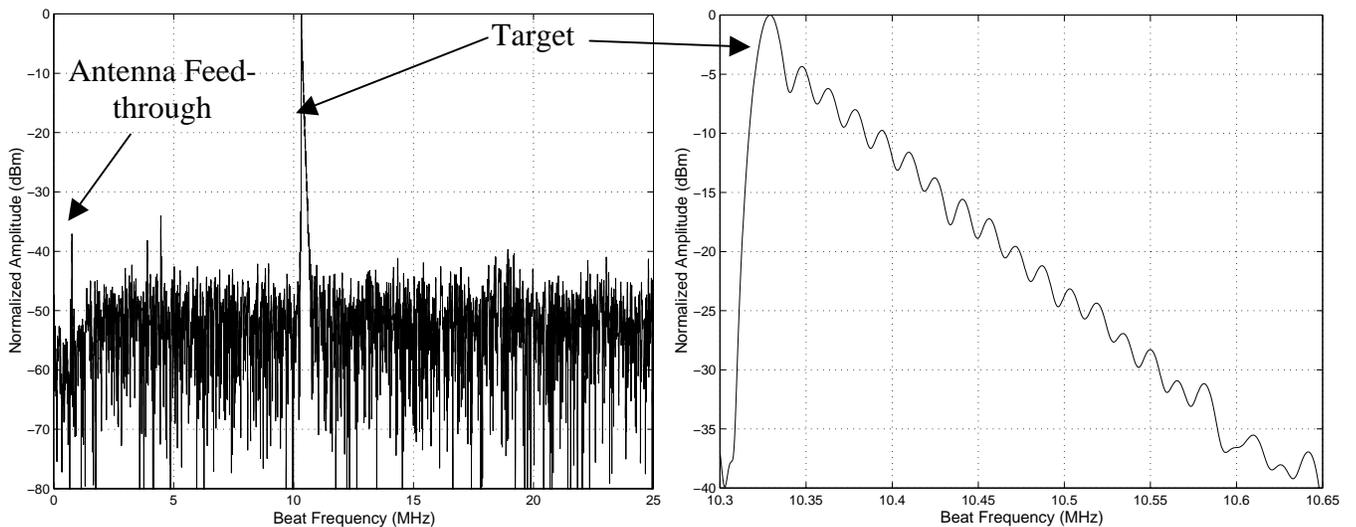
Figure 7.11. Results of FM-CW radar test with target simulator.
