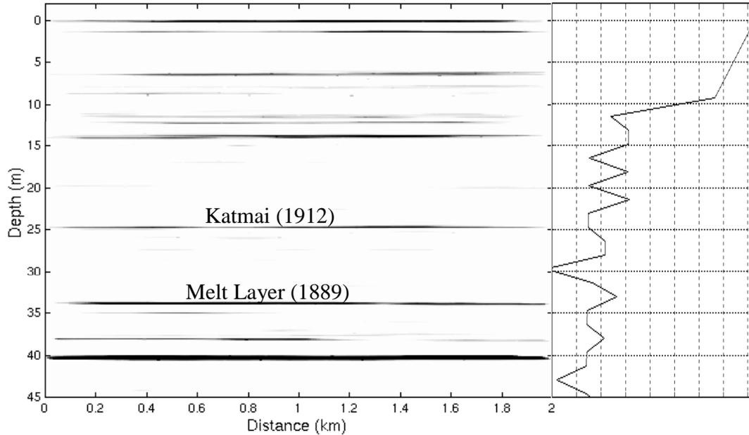
Figure 5.16. Internal layers observed in 1998 (0-45 m depth) compared with reflections due to density changes..
