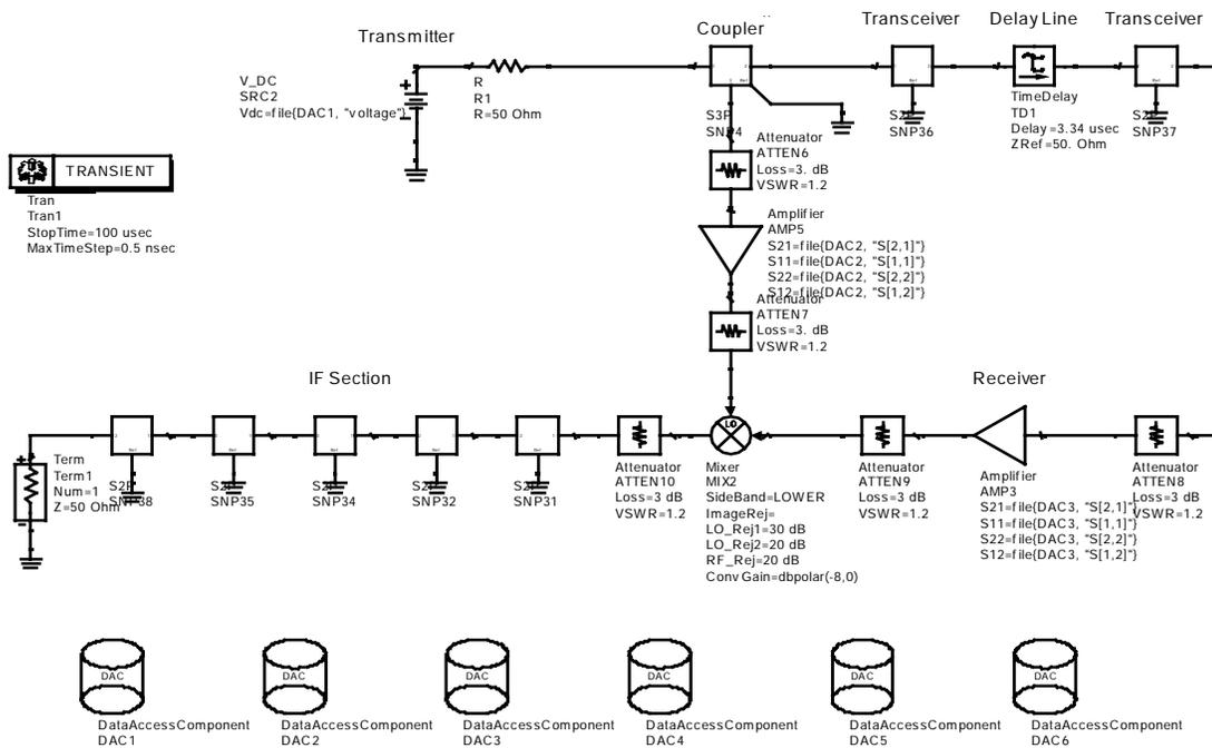
Figure 7.7. FM-CW radar system setup in EEsof®.
