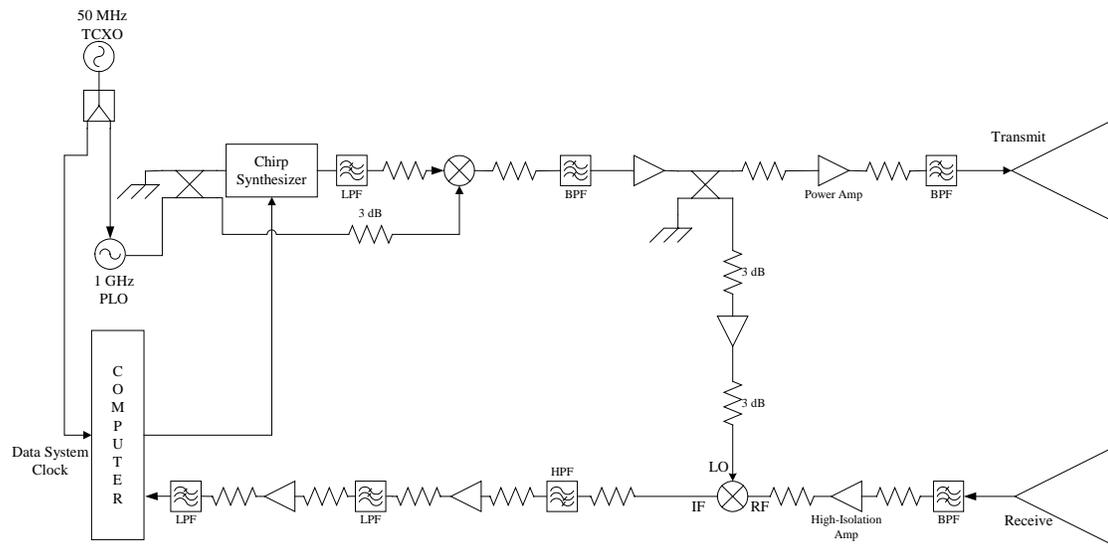
Figure 7.1. Block diagram of improved airborne radar system.
