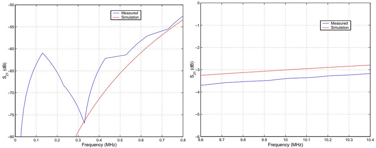
Figure 7.4. A zoom-in of the Gaussian filter's attenuation at 500 kHz (left) and 10 MHz (right).
