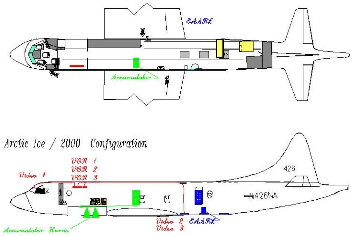
Figure 6.3. Location of accumulation radar and antennas marked in green on NASA's P-3 (courtesy of Doug Young, NASA Wallops).
