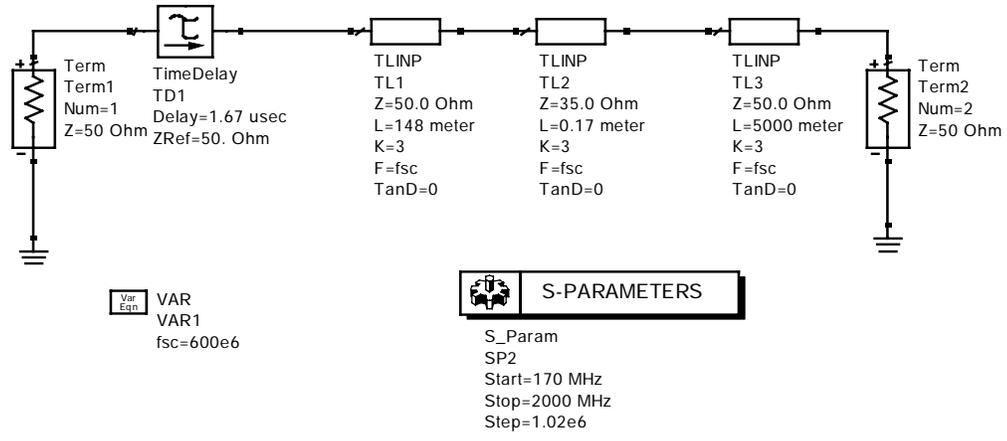
Figure 5.18. EEsof® setup to simulate the effects of finite layer thickness.
