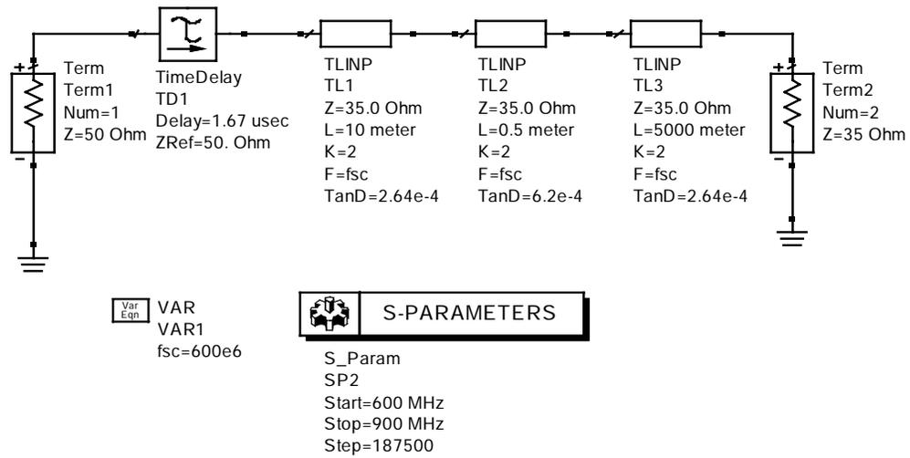
Figure 3.3. Setup on EEsof® to simulate pulse response to layered media.
