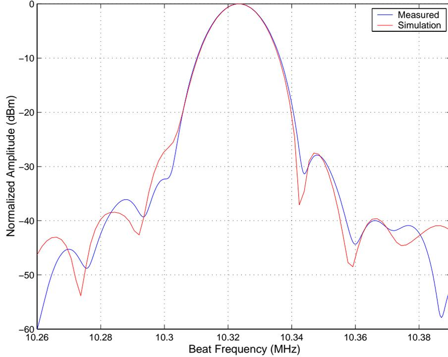
Figure 7.8. Comparison between measured and simulated delay line response.
