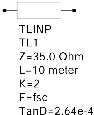
Figure 3.2. Transmission line model in EEsof®.
