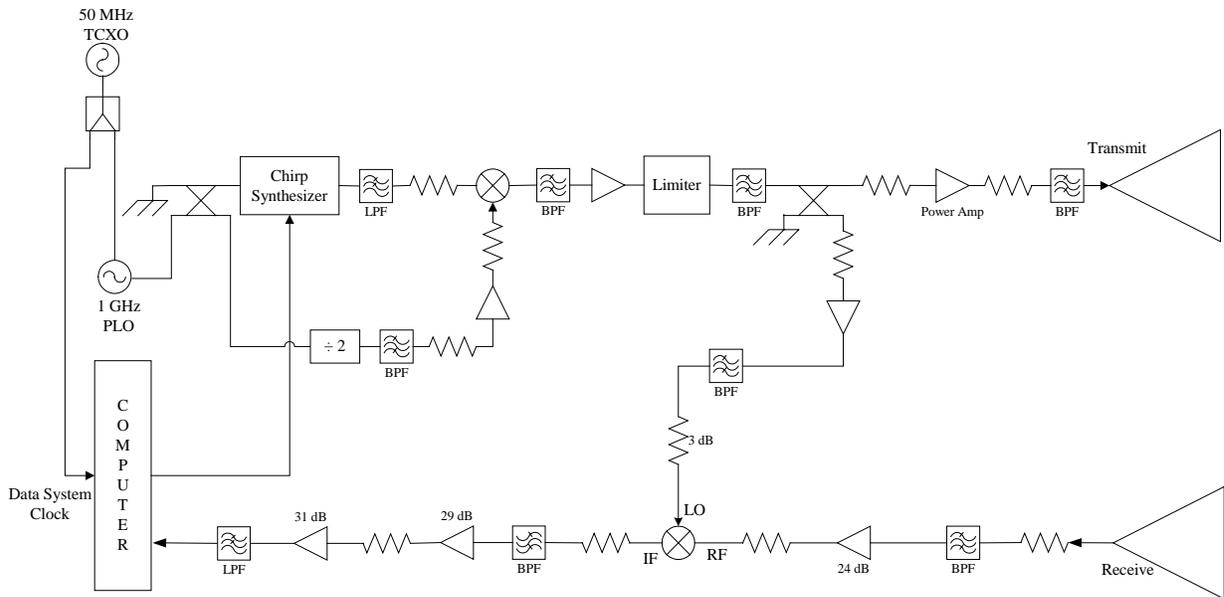
Figure 6.1. Block diagram of the prototype wideband FM-CW radar system for airborne mapping of internal layers.
