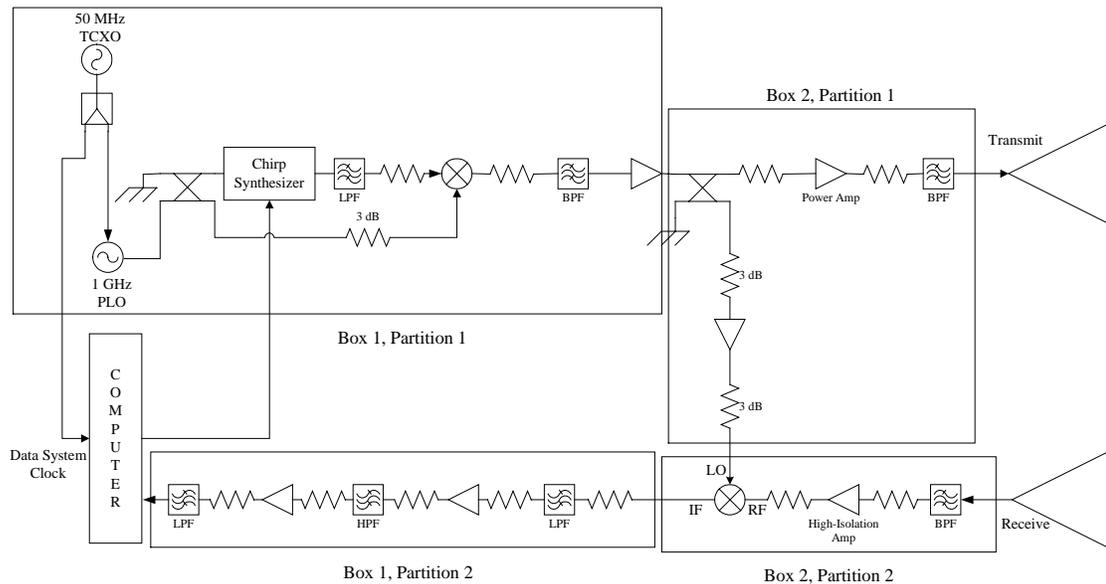
Figure 7.12. Isolating the transmit, receive and IF sections.
