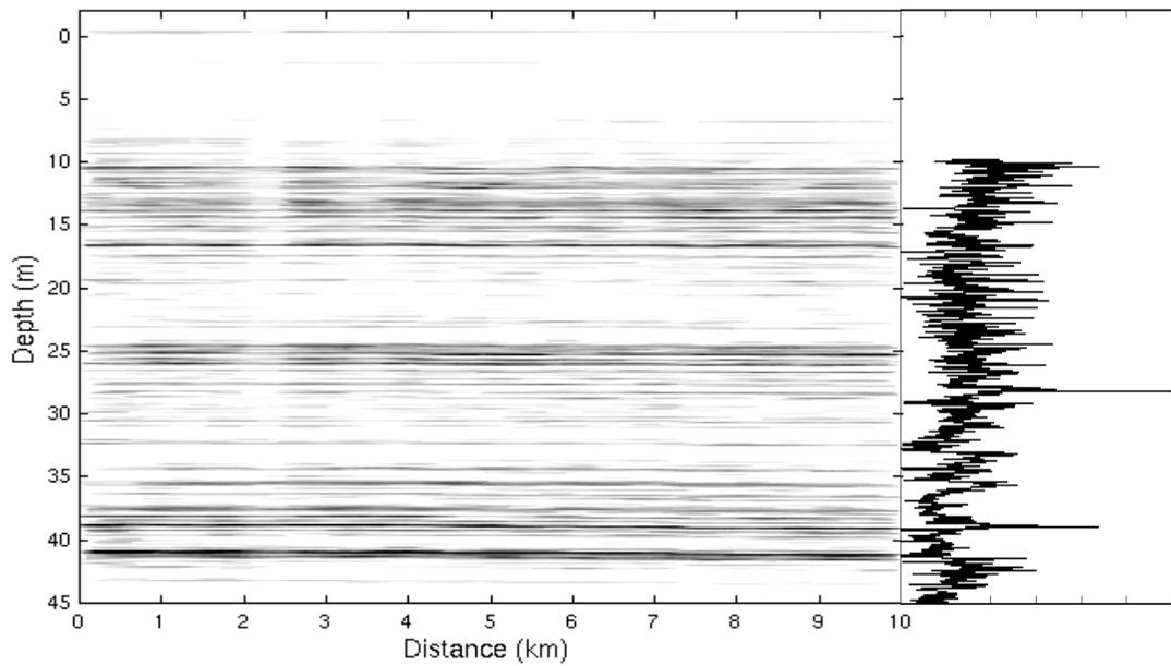
Figure 5.10. Internal layers observed along a 10 km transect in 1999 (0-45 m depth).
