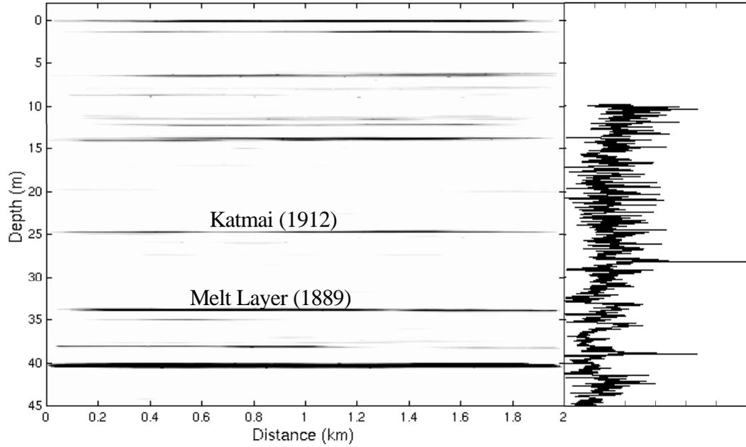
Figure 5.9. Internal layers observed along a 2 km transect in 1998 (0-45 m depth).
