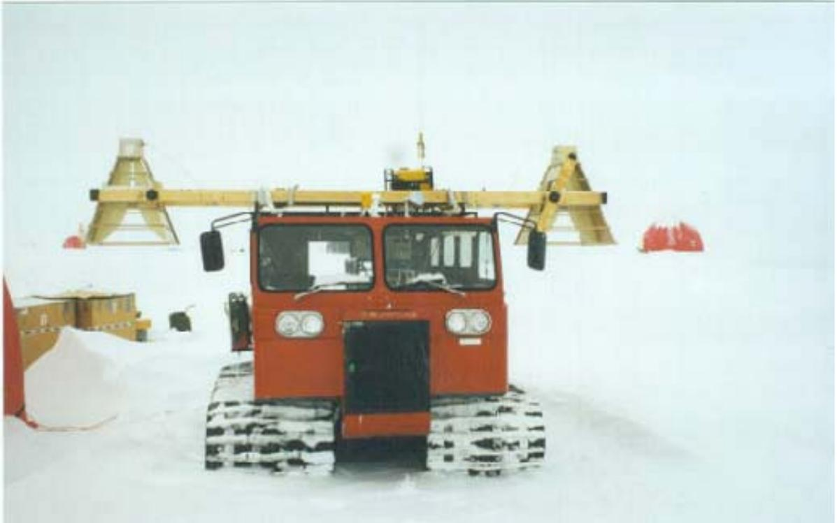
Figure 5.4. Horn antennas mounted on either side of the Trackmaster.
