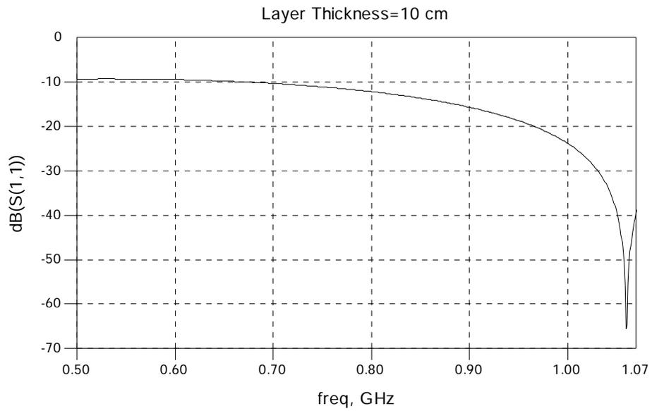
Figure 5.20. Simulated frequency response of reflection from a 10 cm layer.
