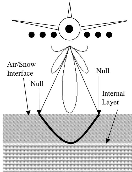
Figure 8.2. Digital beamforming to null out undesired clutter.
