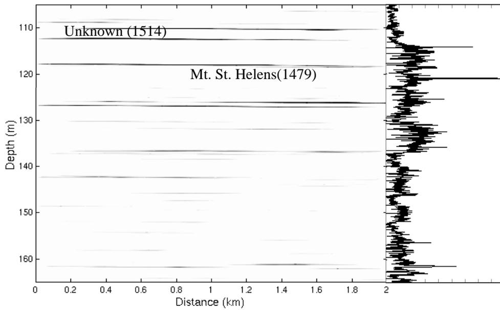
Figure 5.13. Internal layers observed along a 2 km transect in 1998 (105-165 m depth).
