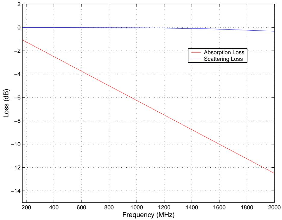
Figure 5.2. Propagation loss through the ice sheet for a distance of 150 m.
