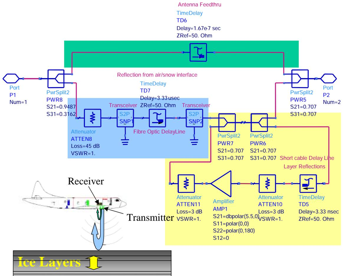
Figure 7.9. Block diagram of target simulator and the effects that are being simulated.
