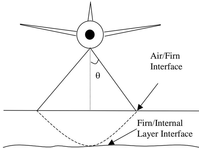
Figure 4.1. Clutter problem in airborne systems. Off-angle surface clutter may mask reflections from deeper layers.
