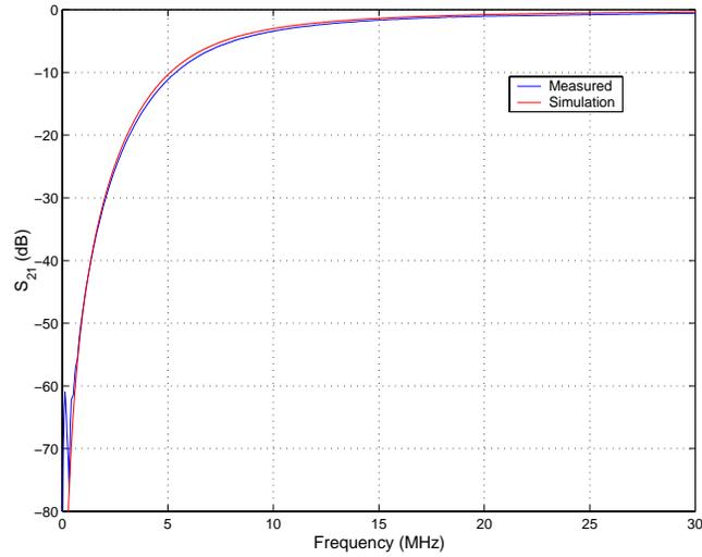
Figure 7.3. Comparison between measured and simulated response of Gaussian high-pass filter.
