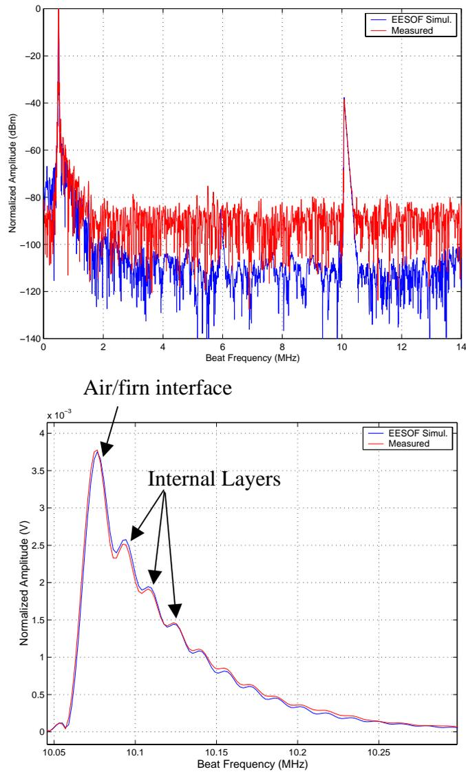
Figure 7.10. Comparison between simulated and measured response of target simulator.
