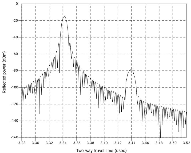
Figure 3.4. Reflection profile of EEsof® simulation. The pulse width of the second reflection is about 1.4 times the reflection from the first interface.
