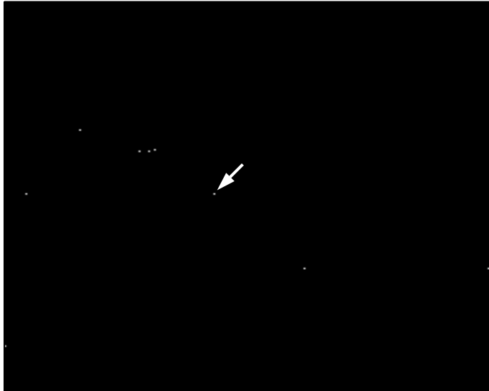
Figure 4-36. The result of applying a threshold to Fig. 4-35. The threshold was set for a P_{fa} of 10^{-6} . The location of the moving target is indicated.
