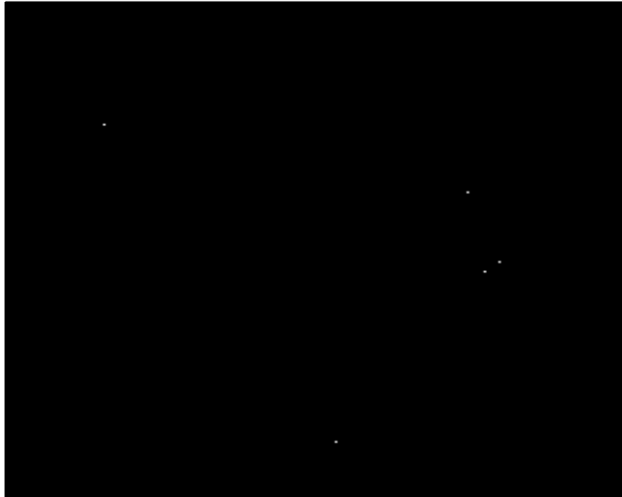
Figure 4-34. The result of applying a threshold to Fig. 4-32. The threshold was set for a P_{fa} of 10^{-6} using the Rayleigh curve fit of Fig. 4-33.
