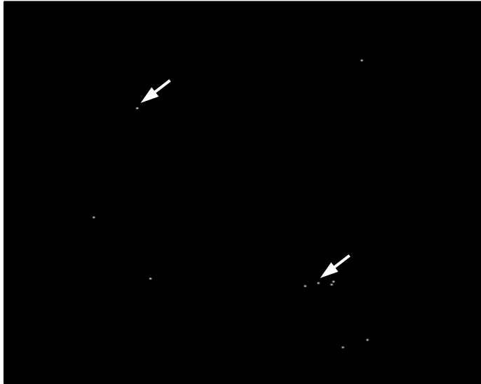
Figure 4-38. The result of applying a threshold to Fig. 4-37. The threshold was set for a P_{fa} of 10^{-6} .
