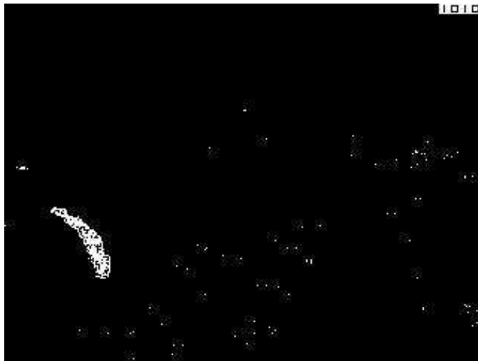
Figure 3.4. Moving pixels segmented after subtraction from average background model and thresholding the difference
