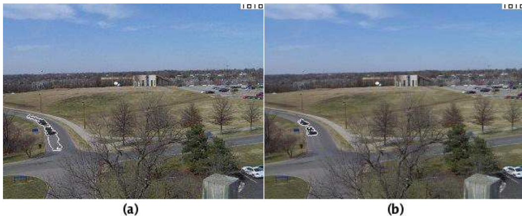
Figure 3.5. (a)Tails due to basic segmentation (b) Corrected results after use of Secondary background(section 3.1.2)
