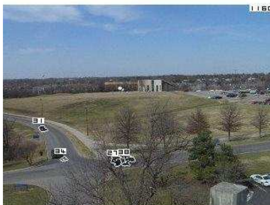
(c) Merge threshold 10 for frame 1160 - Error: Cars 27 and 38 not merged
