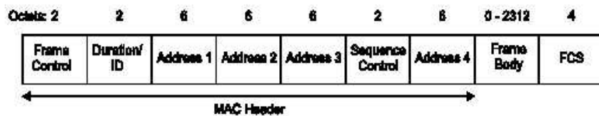
Figure 2.5 802.11 Frame Format Source: 802.11 Specification.
