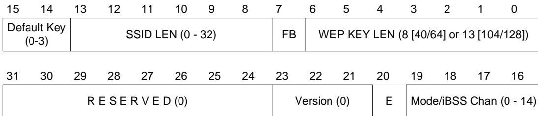
Figure 4.2 Wi-Fi-Co Header Format
