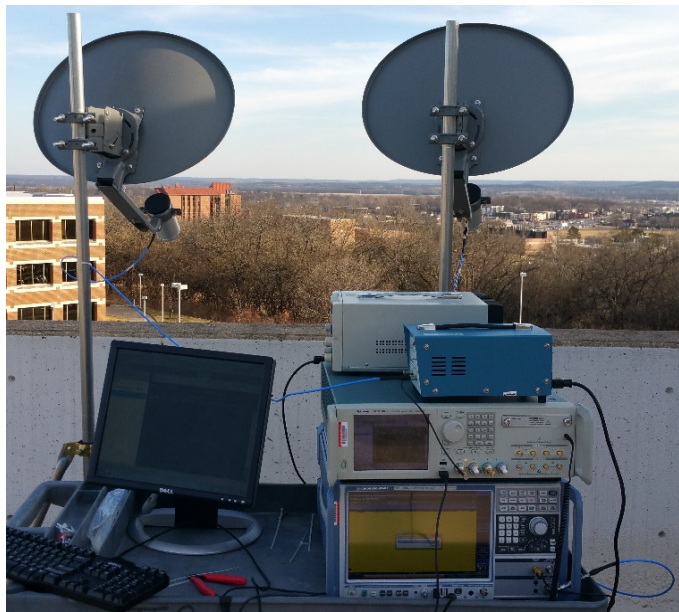
Figure 3.15: Hardware instrumentation setup for open-air measurements
