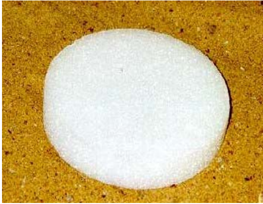
Figure 3.2.1: Picture of the Styrofoam disc used to simulate a mine in the sandpit experiments.
