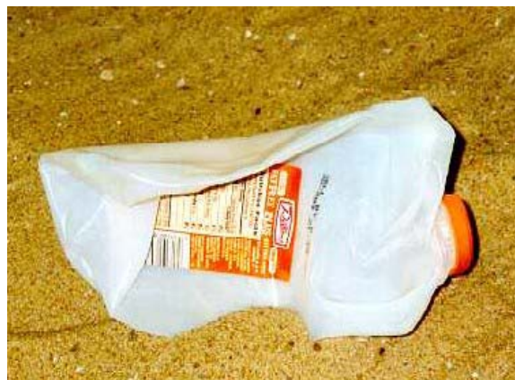
Figure 5.2.1.2: Picture of a crushed milk jug used to simulate a clutter target in the sandpit experiment.
