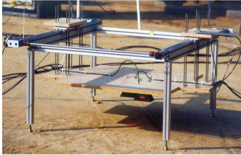
Figure 4.2.2.1: Mobile machine used to collect data by implementing the scans detailed in Figures 4.2.1 and 4.2.2 and thereby simulate the hand-held detector.
