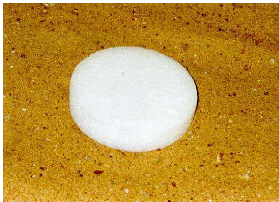
Figure 5.2.1.1: Picture of the Styrofoam disc used to simulate a symmetric landmine in the sandpit experiments.
