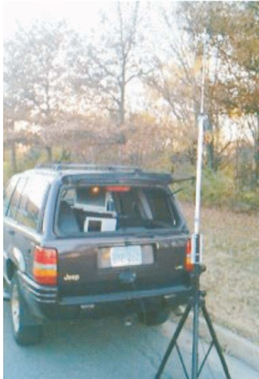
Figure 5.2. Picture of the field measurement setup showing the disc-horn antenna mounted on a tripod stand, laptop and spectrum analyzer (placed inside vehicle).
