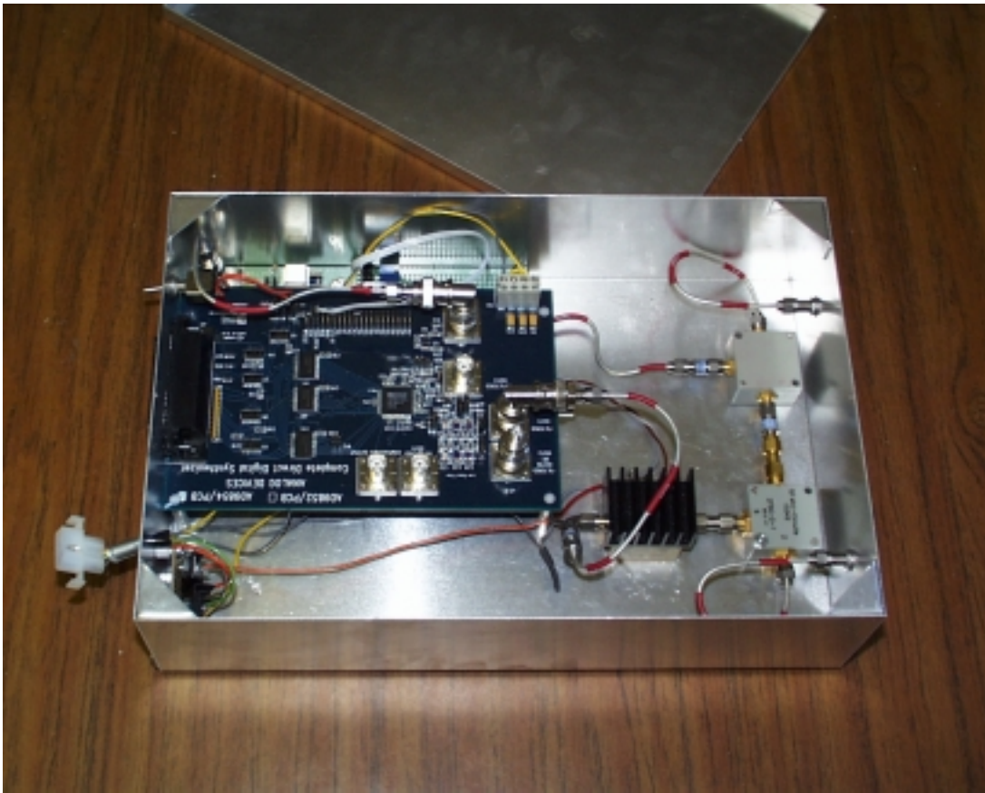
Figure 3-1. Radar system (excluding laptop, batteries, and antennas).
