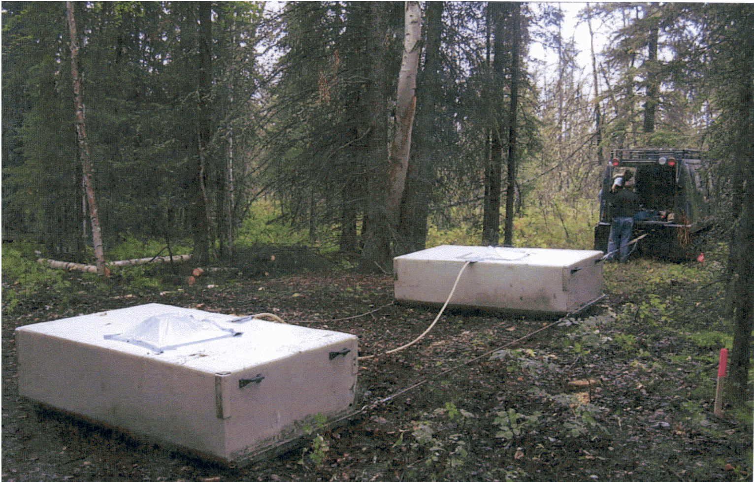
Figure 5-18. GSSI 50 MHz antenna subsystems.
