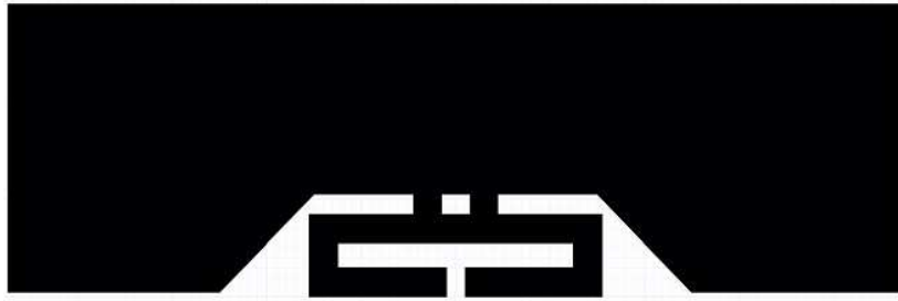
Fig. 4: FCC Planar Microstrip RFID antenna-top view [taken from 12].
