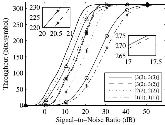
Fig. 2. Throughput results for a multicarrier spatial diversity transceiver employing uniform bit allocation with all antennas active (circle markers), non-uniform bit allocation with all antennas active (triangle markers), uniform bit allocation with antenna subset selection, i.e., variant Var1 (asterisk markers), and non-uniform bit allocation with antenna subset selection, i.e., variant Var3 (no markers). Results are for several antenna/RF chain configurations of  $[N_T(L_T), N_R(L_R)]$ .
