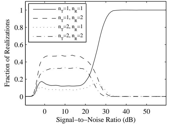
Fig. 3. Fraction of  $[n_T, n_R]$  array configurations occurring for the proposed signal-level antenna subset selection employing non-uniform bit allocation. The transceiver has available  $[N_T = 3, N_R = 3]$  antennas and  $[L_T = 2, L_R = 2]$  RF chains.
