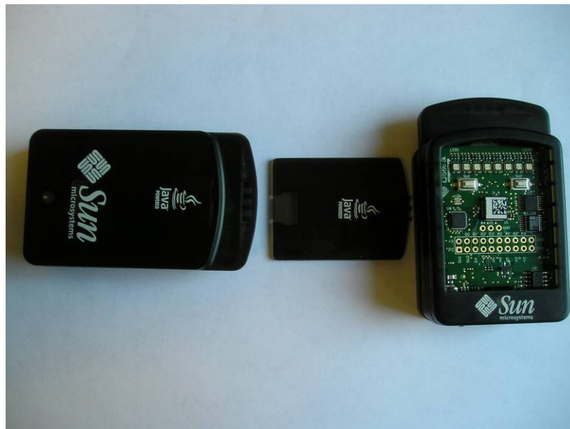
Figure 5: Base station and Free-Range Sun SPOTs
