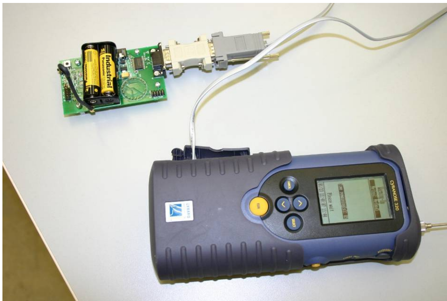
Figure 3: Assembly of MICA2 node with Cyrano 320 sensor
