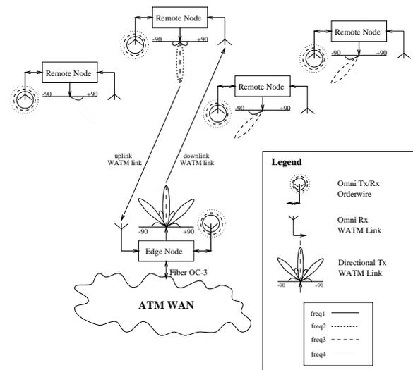
Figure 3: Link-level overview of the RDRN system
