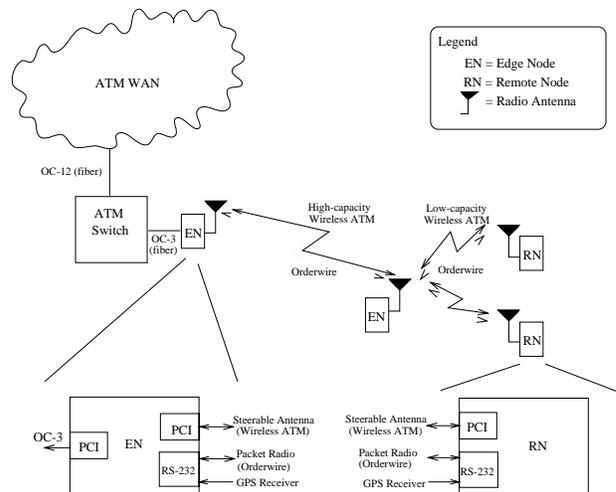
Figure 1: High-level model of the RDRN system
