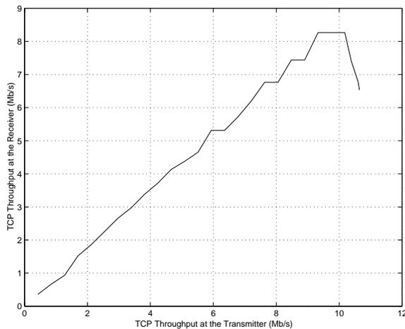
Figure 7: TCP Throughput vs. Transmitted Peak Cell Rate
