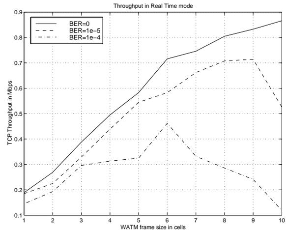
Figure 9: Delay-Sensitive Traffic: TCP Throughput vs. WATM frame size
