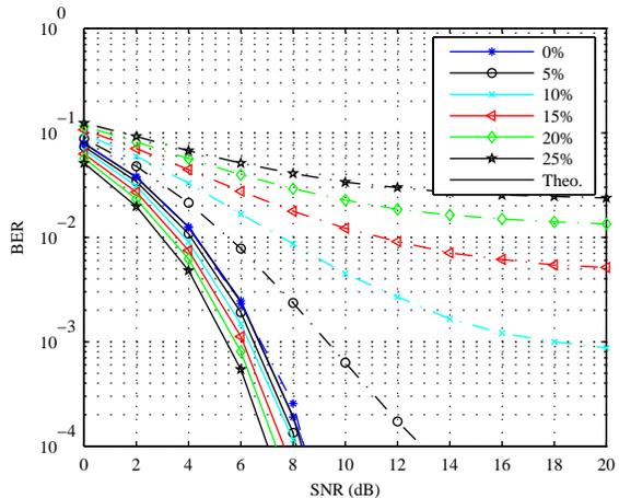
**Fig. 3** BER performance of NC-OFDM (solid lines) and MC-CDMA (dashed lines) transceivers employing  $N = 256$  subcarriers and operating in an AWGN channel.
