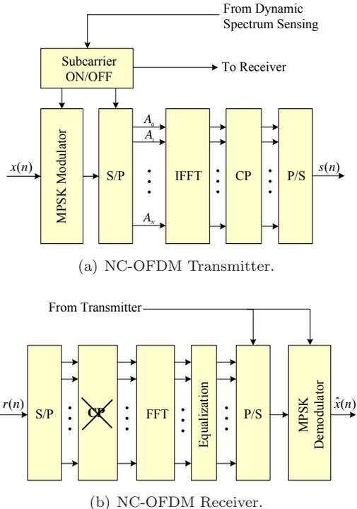
Fig. 1 Schematic of an NC-OFDM transceiver.
