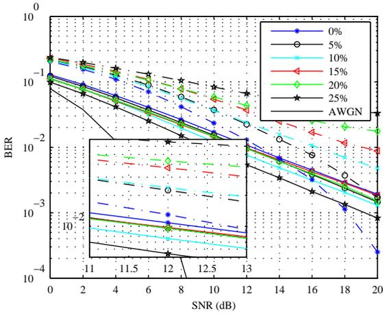
**Fig. 4** BER performance of NC-OFDM (solid lines) and MC-CDMA (dashed lines) transceivers employing  $N = 256$  subcarriers and operating in a 3-path Rayleigh fading channel.
