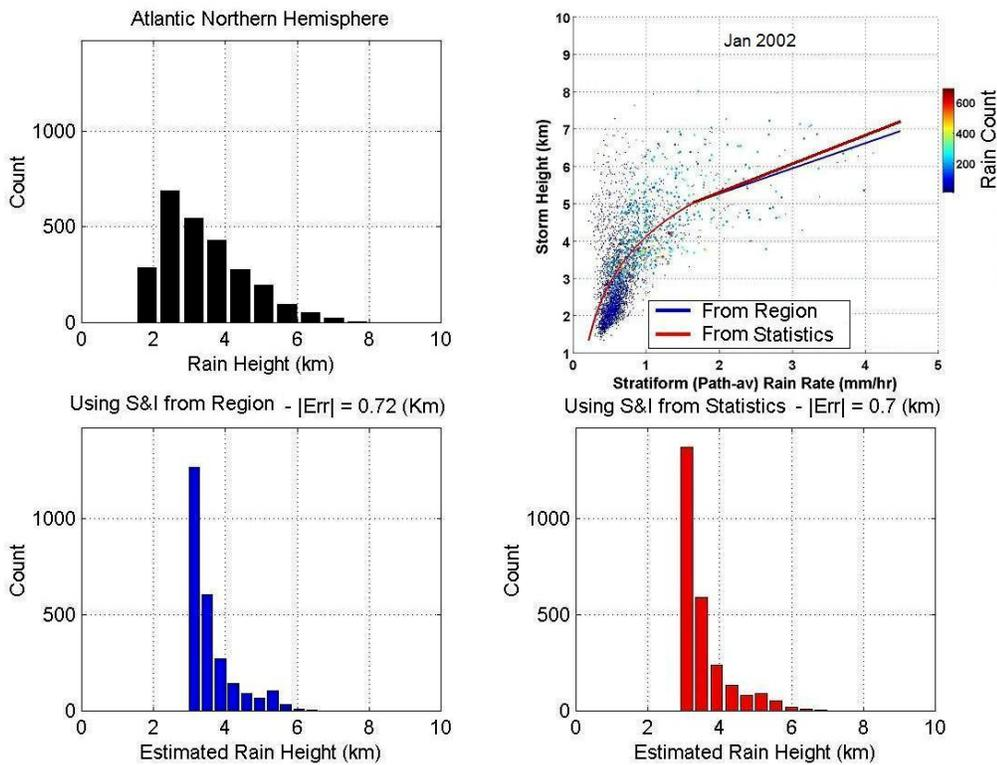
Fig. 7. Comparison of distribution of rain-height estimates obtained from the *Log-Linear Combined* regression fits and from the statistical model.
