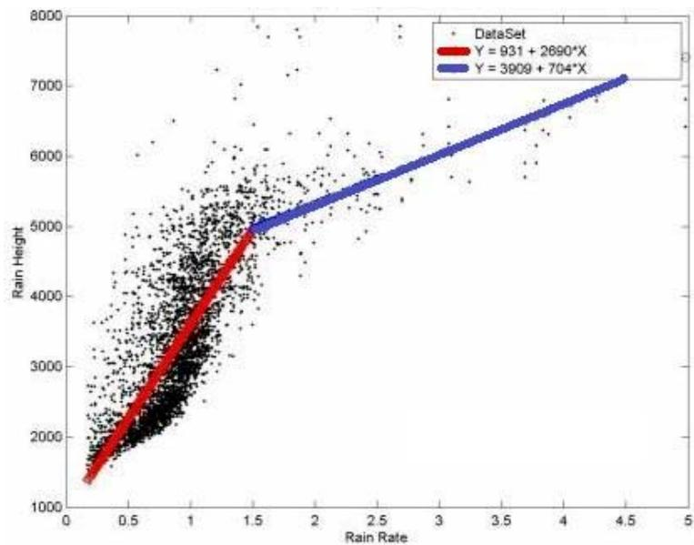
Fig. 2. Bilinear fit for RR vs. RH scatter of stratiform North Atlantic data in January
