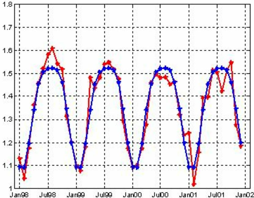
Fig. 5. Seasonal trends of slopes of regression lines for northern-hemisphere convective rain data. Values of slope based on  $\text{Log}(\text{RR})$  vs. RH regression. The red line shows the measured data, and the blue line is the curve from Fourier analysis using the fundamental and two harmonic components.
