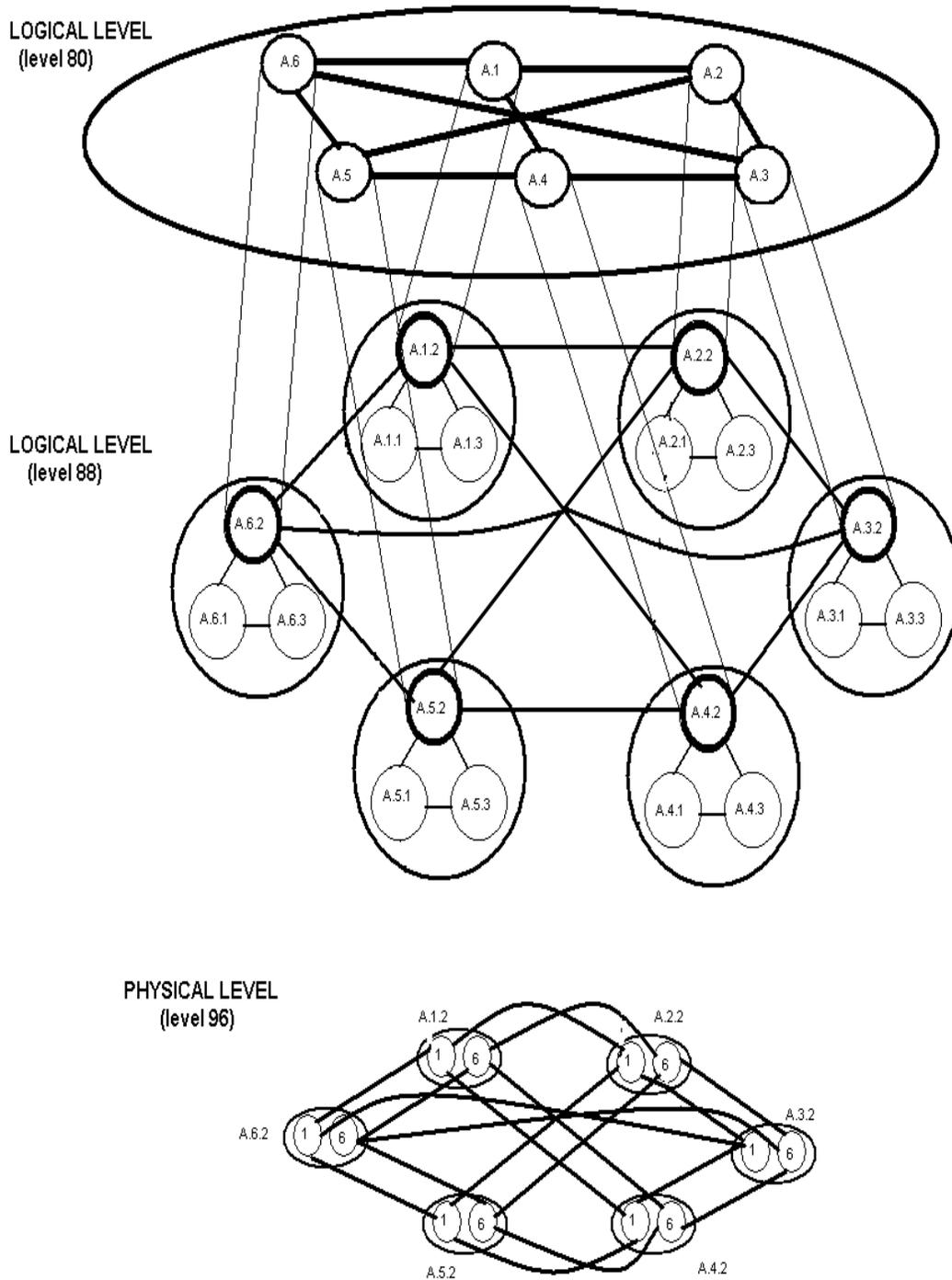
**Fig 6.6 Complete 3-level hierarchical representation of the network**
