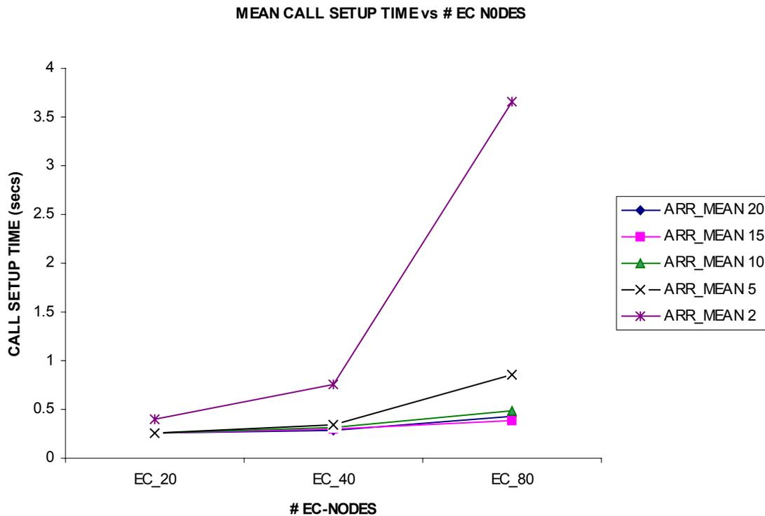
Fig 3.6 Mean Call setup time vs. Topology size
