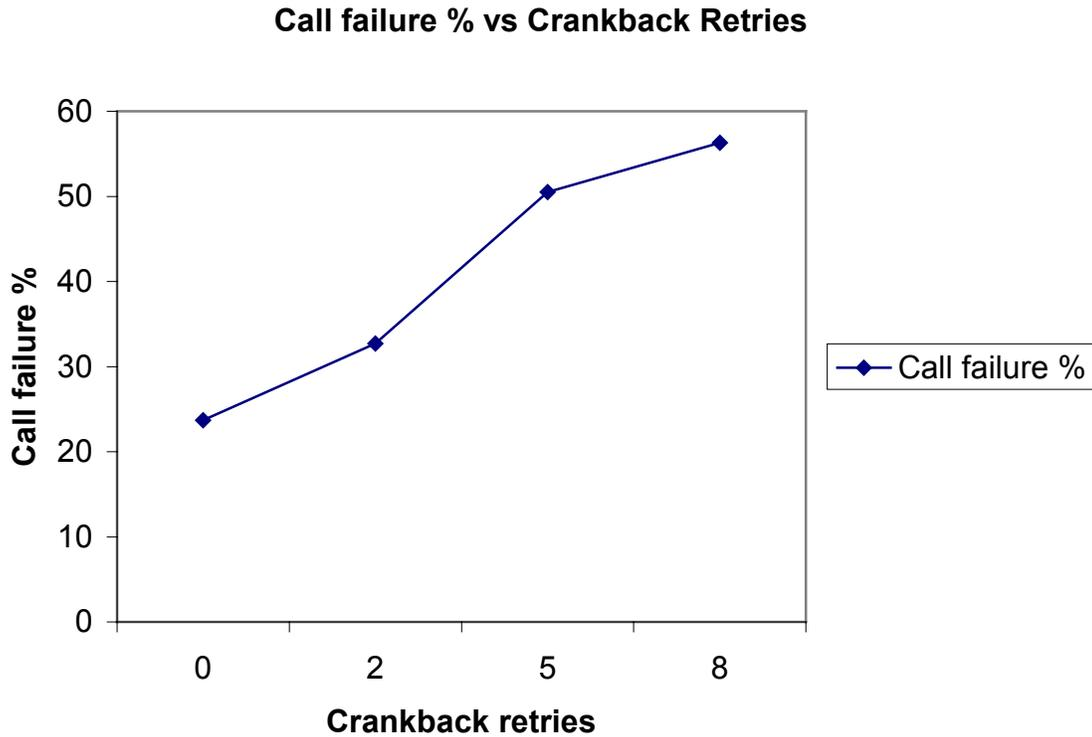
**Fig 7.1 Call failure rate vs. Crankback retries**
