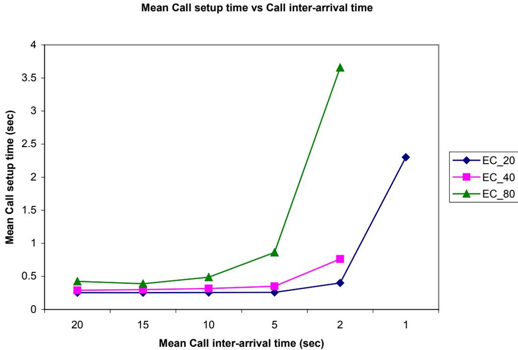
**Fig 4.1 Mean Call setup time vs. Load**
