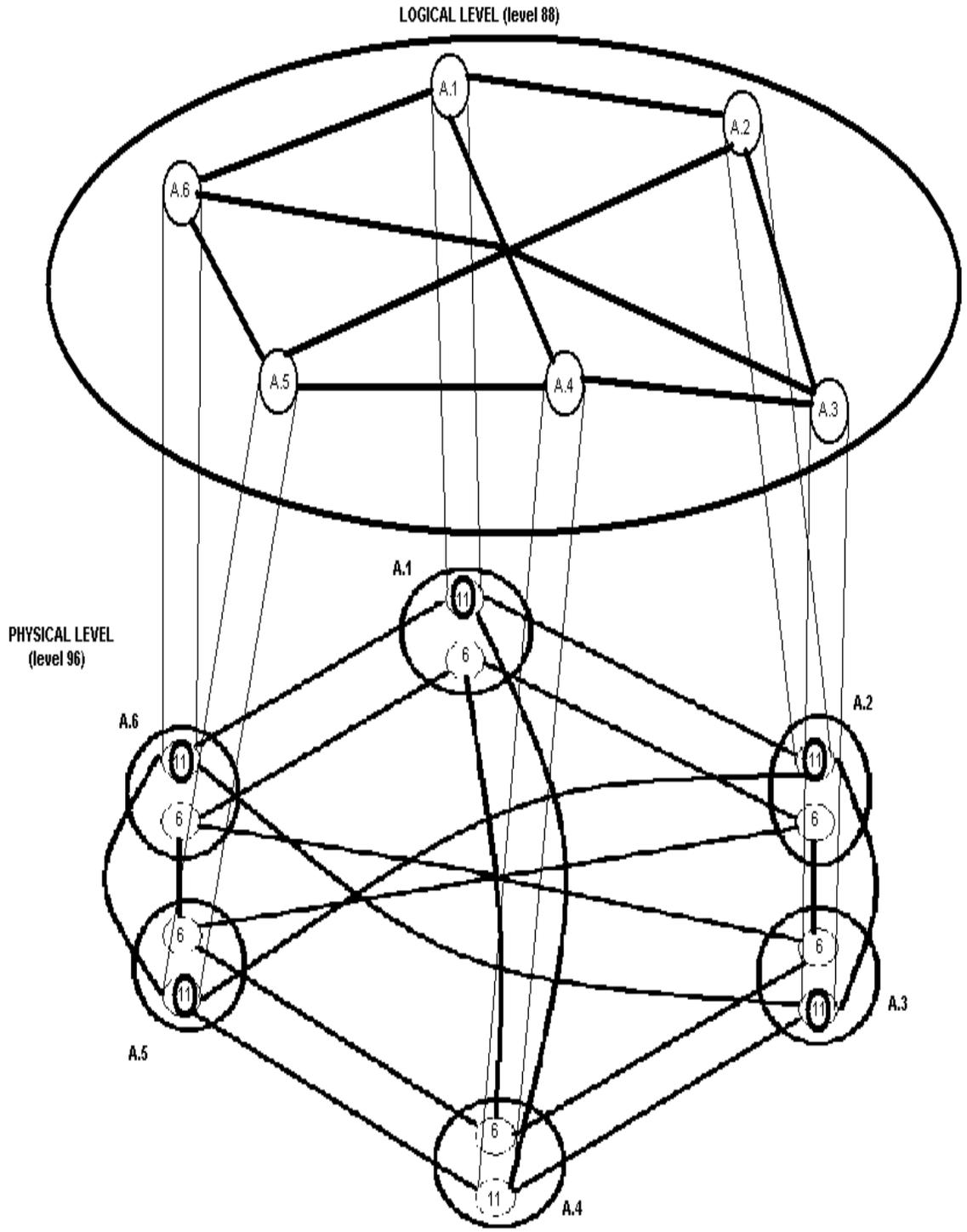
**Fig 6.4 Inter-Peergroup connections in a 2-level hierarchical network**
