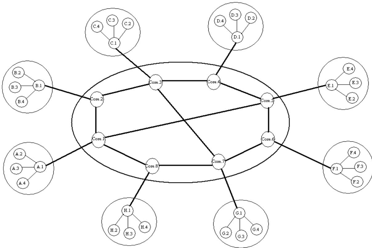
**Fig 3.2 Edge-Core 40 nodes**
