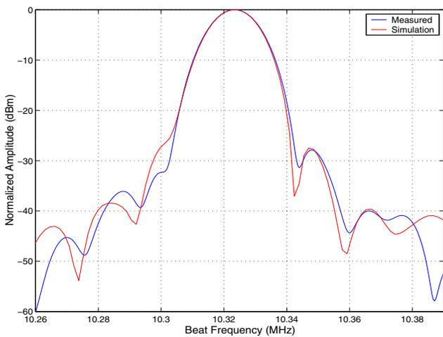
Fig. 3. Comparison between measured and simulated delay line response.
