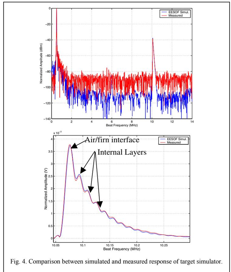
Fig. 4. Comparison between simulated and measured response of target simulator.
