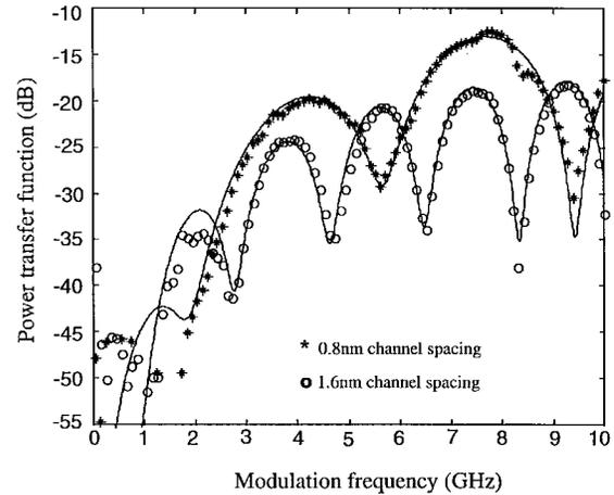
Fig. 3. XPM frequency response in the system with two spans (114 and 116 km) of nonzero dispersion shifted fiber. Stars: 0.8-nm channel spacing ( $\lambda_{\text{probe}} = 1559$  nm and  $\lambda_{\text{pump}} = 1559.8$  nm). Open circles: 1.6-nm channel spacing ( $\lambda_{\text{probe}} = 1559$  nm and  $\lambda_{\text{pump}} = 1560.6$  nm). Continuous lines are corresponding theoretical results.
