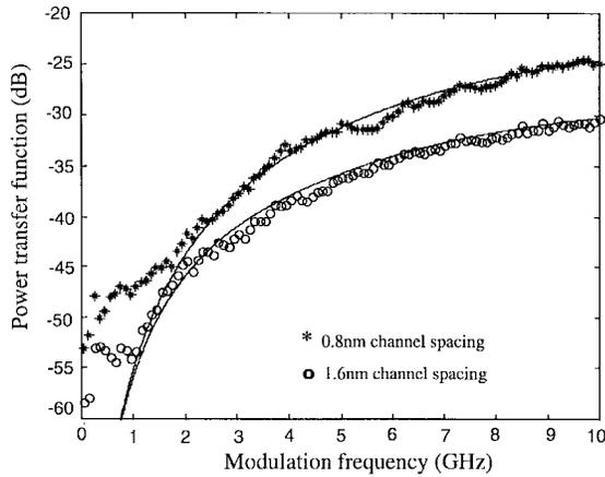
Fig. 2. XPM frequency response in the system with single span (114 km) nonzero dispersion shifted fiber. Stars: 0.8-nm channel spacing ( $\lambda_{\text{probe}} = 1559$  nm and  $\lambda_{\text{pump}} = 1559.8$  nm). Open circles: 1.6-nm channel spacing ( $\lambda_{\text{probe}} = 1559$  nm and  $\lambda_{\text{pump}} = 1560.6$  nm). Continuous lines are corresponding theoretical results.
