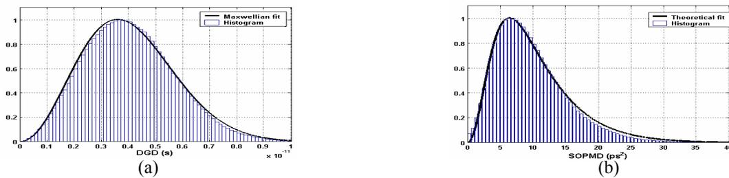
Fig. 1 Probability densities of the magnitude of (a) first-order PMD  $|\vec{\Omega}(\omega)|$ , (b) second-order PMD  $|\vec{\Omega}_\omega|$
