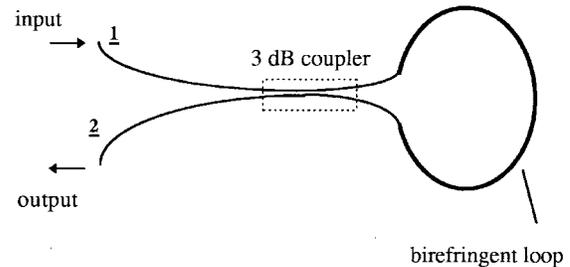
Fig. 1. A Sagnac interferometer with a loop birefringence element.
