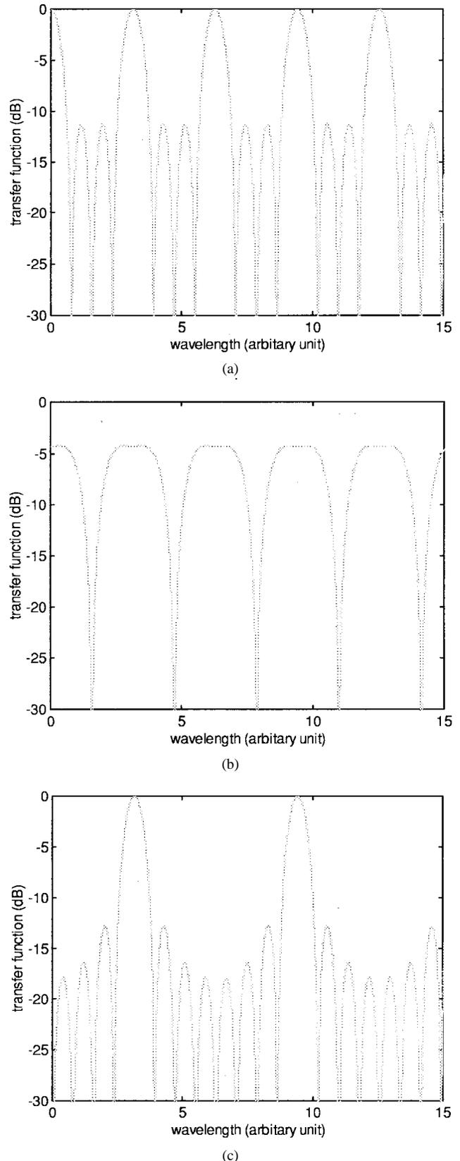
Fig. 3. Calculated intensity transfer functions. (a) First-order Lyot-Sagnac filter. (b) First-order Lyot-Sagnac filter after 1.1 rad of birefringence rotation. (c) Cascade of filters of Fig. 2(a) and Fig. 3(a).
