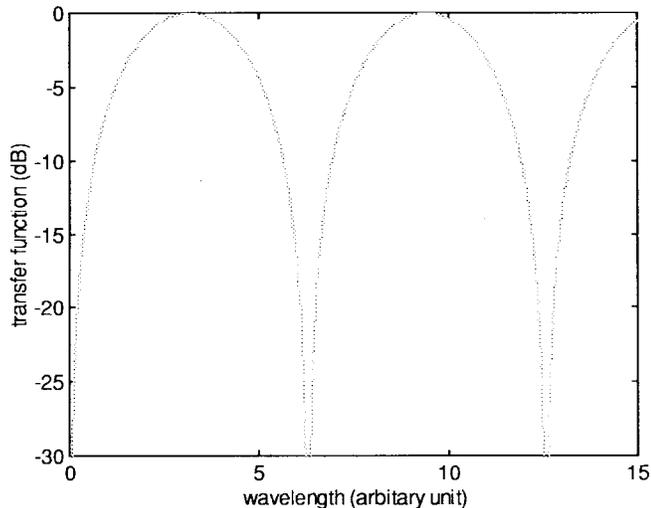
Fig. 2. Calculated intensity transfer functions of the first-order Solc-Sagnac filter.
