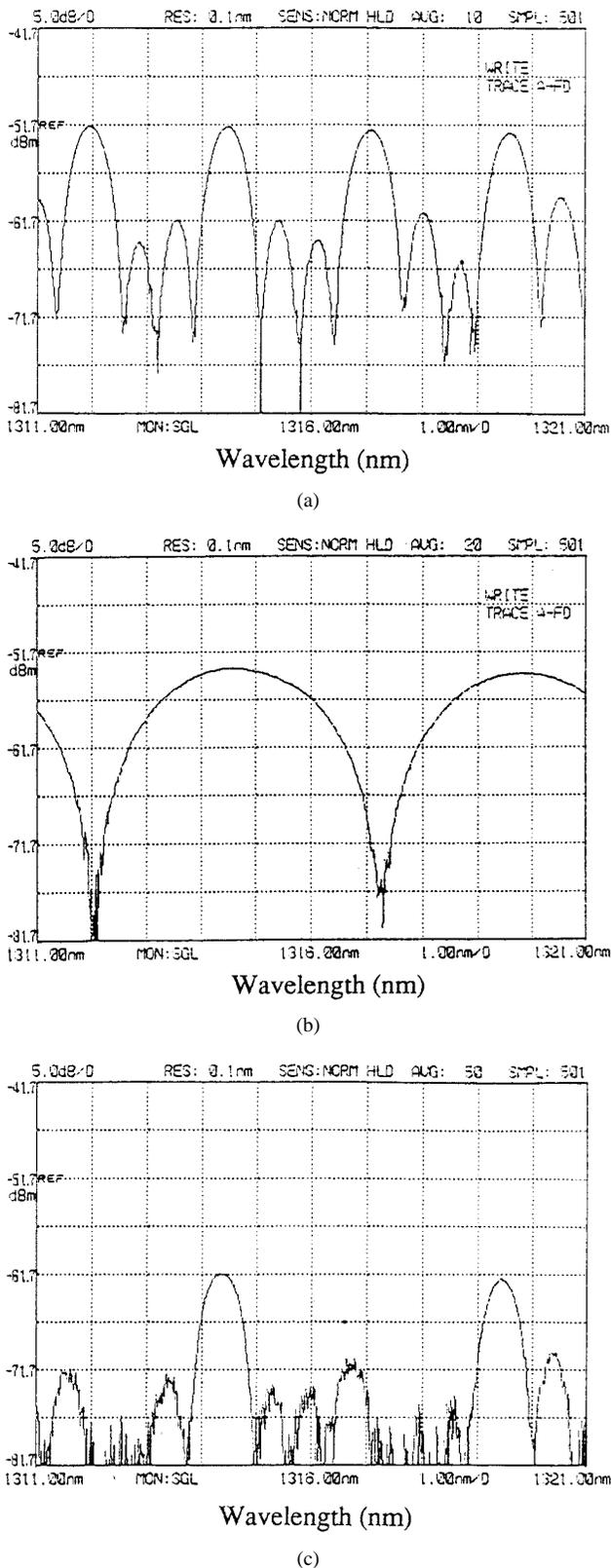
Fig. 4. Measured intensity transfer functions. (a) The first-order Lyot-Sagnac filter. (b) The first-order Solc-Sagnac filter. (c) Two filters in tandem.
