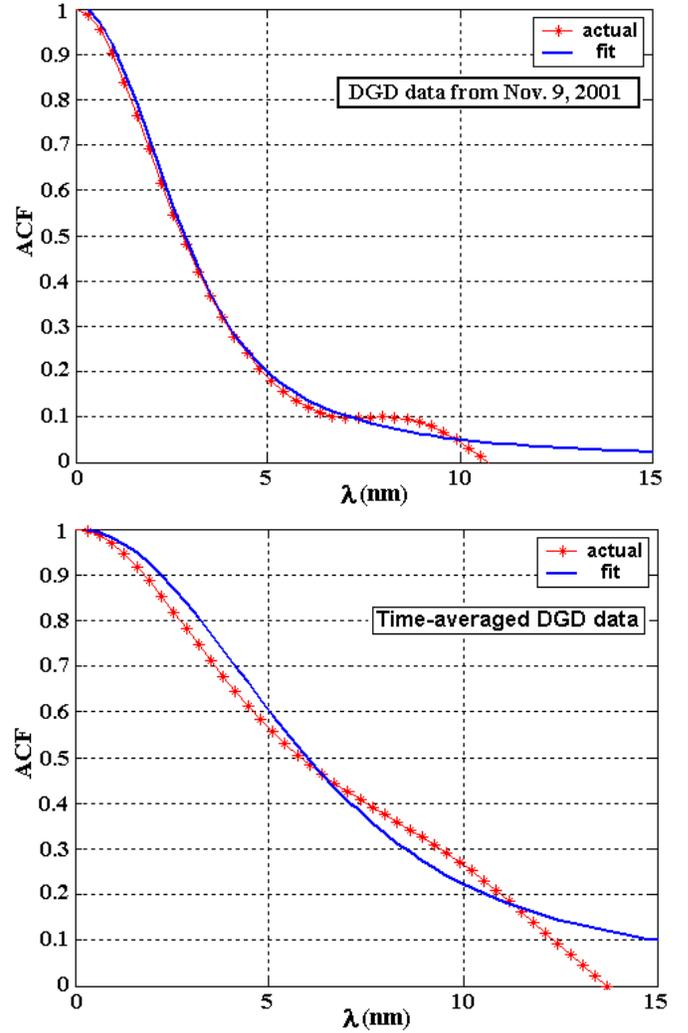
**Figure 7. Normalized spectral autocorrelation functions (ACFs) of normalized DGD data measured (top) on Nov. 9, 2001 and (bottom) time-averaged over all 692 measurements. Theoretical ACF curves are fitted to the measured spectral ACFs.**
