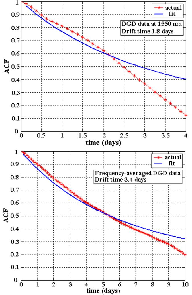
**Figure 5. Normalized temporal autocorrelation functions (ACFs) of normalized DGD data measured (top) at 1550 nm and (bottom) across 1150 frequencies. Theoretical ACF curves are fitted to the measured temporal ACFs.**
