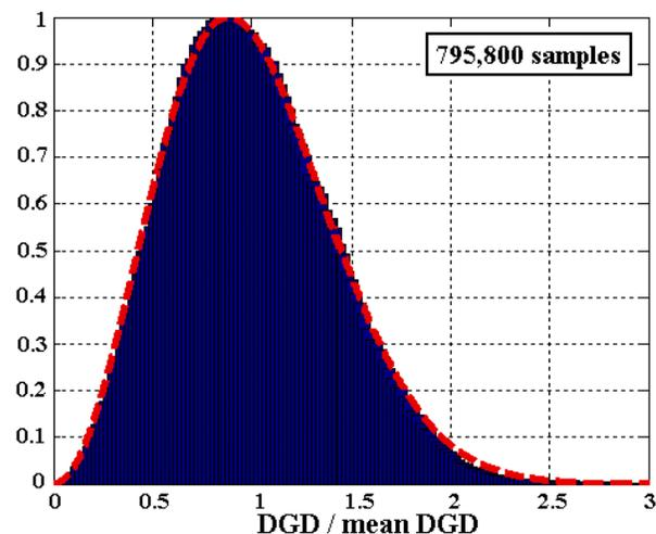
Figure 3. Normalized histogram of measured DGD data.
