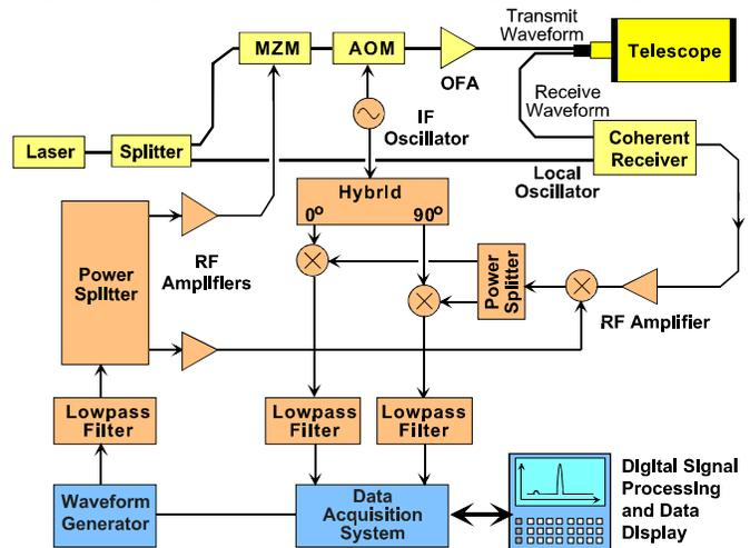
Figure 1. Block diagram of the hybrid RF/laser radar with I and Q direct downconversion. MZM: Mach-Zehnder modulator, AOM: acousto-optic modulator, OFA: optical fiber amplifier.
