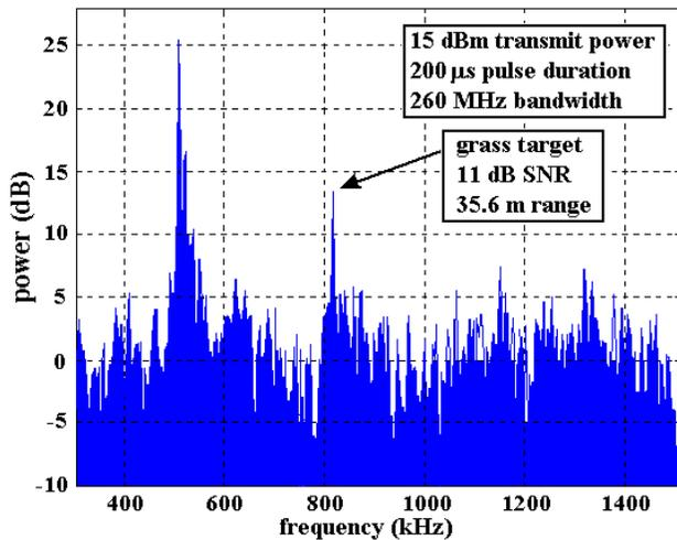
Figure 2. Measured signal from grass. No coherent integrations, no incoherent integrations.
