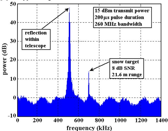
Figure 3. Measured signal from snow surface. No coherent integrations, 100 incoherent integrations.
